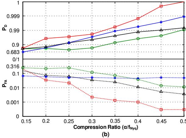
Figure 3. Sub-Nyquist MSS  $P_D$  and  $P_{FA}$  for various compression ratios;  $SNR = 0$  dB. (a)  $T_{ST} = 15\mu s$  and (b)  $T_{ST} = 3\mu s$ .
