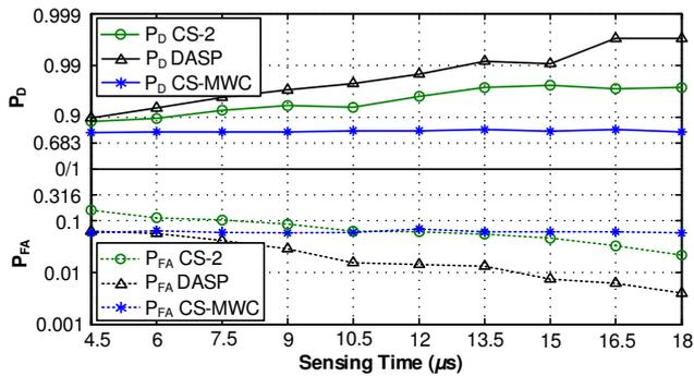
Figure 4. Sub-Nyquist MSS  $P_D$  and  $P_{FA}$  for various sensing time values;  $\alpha/f_{Nyq} = 0.15$  and  $SNR = 0$  dB.
