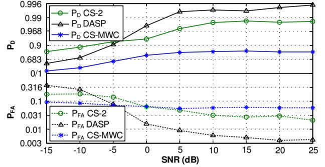
Figure 5. Sub-Nyquist MSS  $P_D$  and  $P_{FA}$  for various  $SNR$  values;  $\alpha/f_{Nyq} = 0.15$  and  $T_{ST} = 15\mu s$ .
