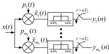
Figure 2. MWC sampler block diagram.
