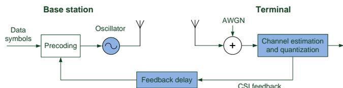
Fig. 1. Sources of imperfect channel knowledge are colored blue: channel estimation and feedback quantization at the terminal, channel aging during the feedback delay and individual synchronization parameters of the base stations.
