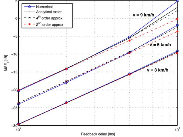
Fig. 3. MSE due to channel aging according to numerical evaluation and exact analytic expression (10), second and fourth order approximation (14).
