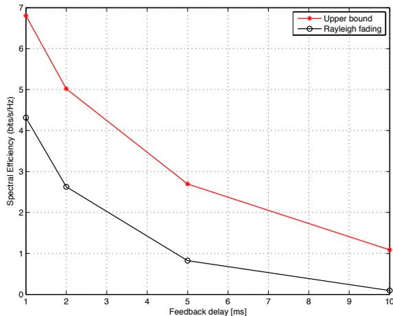
Fig. 5. Spectral efficiency for JT CoMP with ZF precoding under the presence of channel aging and synchronization errors. Parameters are given in Table I.
