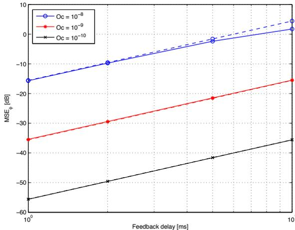
Fig. 4. Equivalent channel MSE due to oscillator CFO. *solid*: numerical evaluation of exact expression (21); *dashed*: analytical approximation (24).
