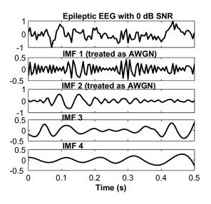
Fig. 8. The four IMFs of the epileptic signal with 0 dB SNR.
