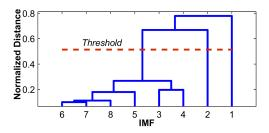
**Fig. 6**. The dendrogram and threshold for normal EEG recording with 0 dB SNR.
