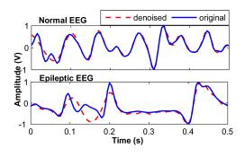
Fig. 9. Reconstruction of EEG signals with 20 dB AWGN.
