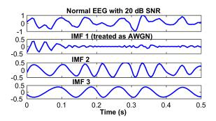
Fig. 4. The three IMFs of the normal EEG with 20 dB SNR.
