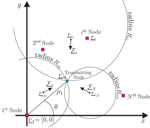
**Fig. 2.** Focussing vectors and loci used for localization in  $\mathcal{R}^2$  space.  $\mathcal{F}_i$  represents the  $i^{\text{th}}$  focussing vector.
