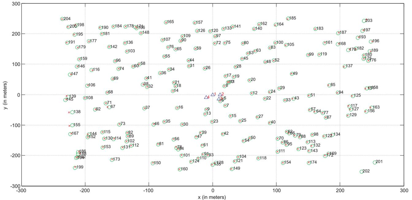
**Fig. 3.** Sequential discovery with target nodes having a coverage of  $D = 100\text{m}$  with  $\text{SNR} = 30\text{dB}$ . Node locations are averaged over  $K = 10$  localization attempts. Green circles represent actual node locations, blue triangles represent anchor nodes at known locations, and red crosses represent location estimates. All but nodes 201 and 202 are localized. Location uncertainties can be seen more predominantly at the edges of the network.
