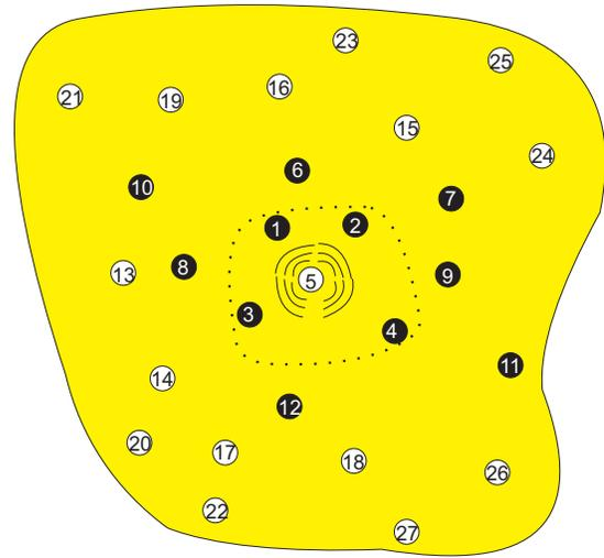
**Fig. 1.** A sequential discovery process. Black nodes are at known or previously estimated locations. Transmitting node 5 is localized using nodes 1, 2, 3 and 4.
