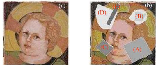
Figure 3: Replica of St. Christopher artwork (a); Defects introduced during its manufacture (b).
