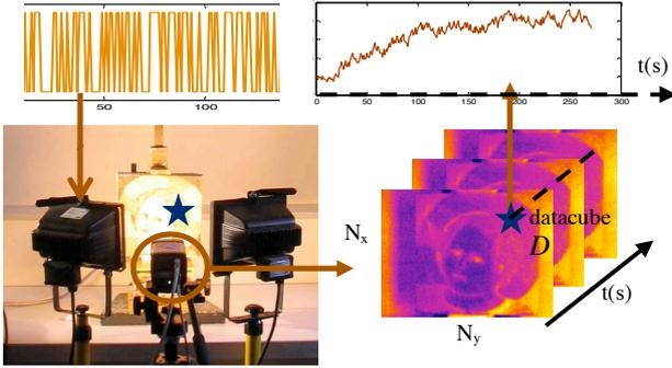
Figure 1: Data acquisition system. Top: excitation and sample of a recorded signal. Bottom right: recorded datacube  $D$ .
