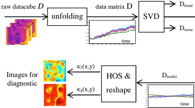
Figure 2: Proposed scheme based on the SVD and HOS of IR response at PRBS random excitations for nondestructive investigation of artworks.
