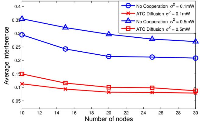
Figure 4: Average interference perceived by the swarm at convergence, for the non cooperative estimation case and for adaptive diffusion.
