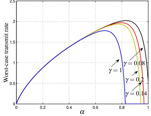
Figure 4: Worst-case transmit rate versus  $\alpha$  for different values of the dynamic range  $\gamma$ .
