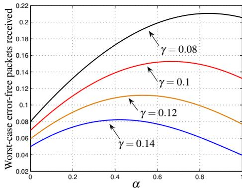
Figure 6: Worst-case number of error-free packets received per frame versus  $\alpha$  for different values of the dynamic range  $\gamma$ .
