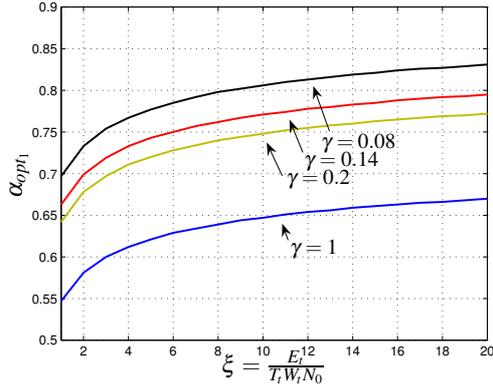
Figure 5: Optimum value of  $\alpha$  for the maximization of the worst-case transmit rate versus  $\xi$  for different error scenarios.
