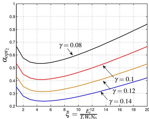
Figure 7: Optimum value of  $\alpha$  for the maximization of the worst-case number of error-free packets received per frame versus  $\xi$ .
