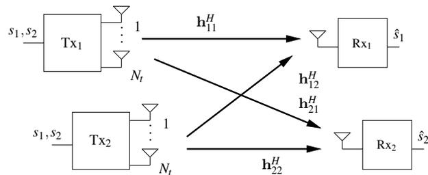
Figure 1: System model of a coordinated scheme in flat fading channels where both transmitters communicate simultaneously toward both receivers.
