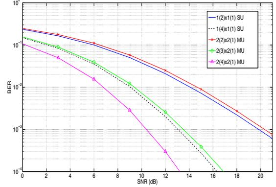
Figure 2: displays the BER curves versus the SNR of the considered ZF beamforming scheme, i.e., the multi-user (MU) scenario, with  $N_t = 2$ ,  $N_t = 3$  and  $N_t = 4$  assuming perfect frequency synchronization and for a 16QAM modulation scheme. The BER curves of a single-user (SU) system with transmit-MRC beamforming and  $N_t = 2$  and  $N_t = 4$  are also displayed.
