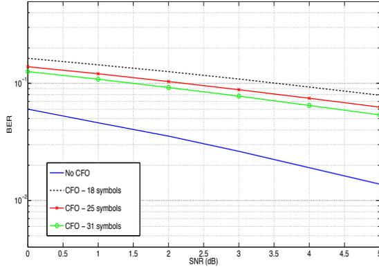
Figure 3: displays the BER curves obtained for a BPSK modulation scheme,  $f_{\Delta} = 2\text{ppm}$  and for 18, 25 and 31 transmit symbols ( $T_p$ ). These values represent the minimum, a zero and a local maximum of the  $\text{sinc}(2\pi f_{\Delta} T_p)$  function. The curve of the SNR gain without CFO is also displayed.
