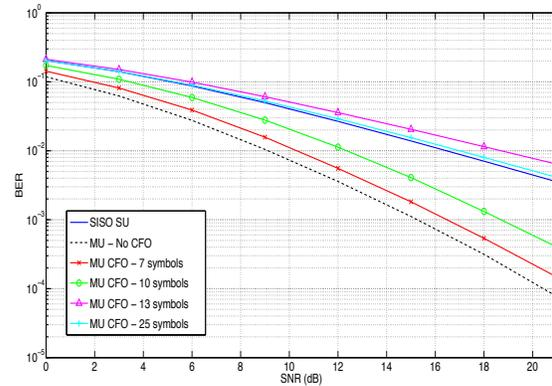
Figure 4: shows the BER curves for various transmission durations based on the derivations in Section 4.3. The simulations are for  $f_{\Delta} = 2\text{ppm}$  and a 4-QAM modulation scheme
