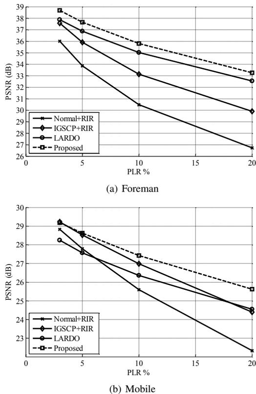
Figure 4: PSNR vs. Packet loss rate for different methods for (a) Foreman sequence and (b) Mobile sequence with QCIF size and 15 fps at 256 kbps.
