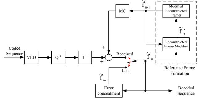
Figure 2: Block diagram of a video decoder with reference frame modification.
