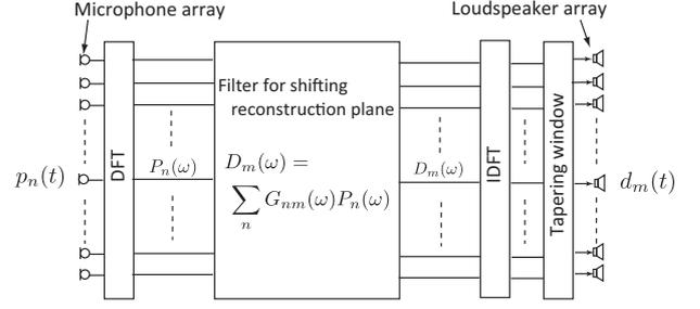
Figure 3: Block diagram of practical system for shifting reconstruction plane.
