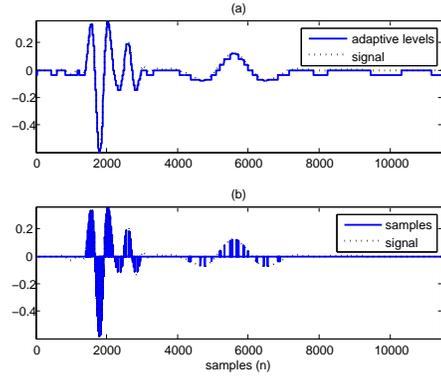
Figure 6: Adaptive LC of a bursty signal: (a) quantization with local means, (b) times of local averages.
