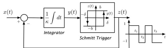
Figure 1: Asynchronous sigma delta modulator
