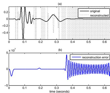
Figure 9: (a) PSWF reconstruction from uniform levels and their times, (b) reconstruction error.
