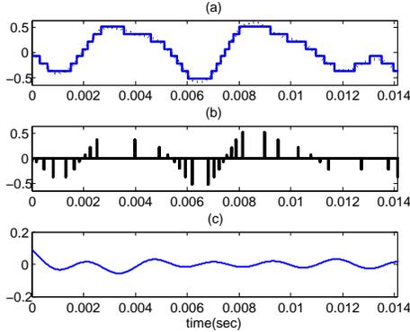
Figure 5: Uniform LC sampling ((a) and (b)) and reconstruction error (c) of a smooth signal.
