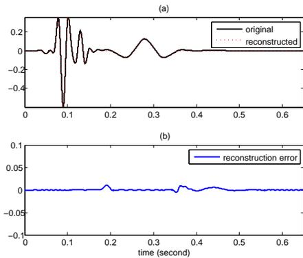
Figure 7: (a) PSWF reconstruction from local levels and their times, (b) reconstruction error.
