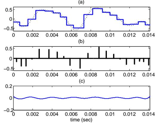
Figure 4: Adaptive LC sampling ((a) and (b)) and reconstruction error (c) of a smooth signal.
