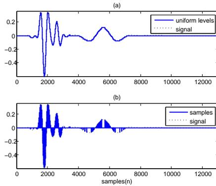
Figure 8: Uniform LC of a bursty signal: (a) quantization with uniform levels, (b) times of uniform levels.
