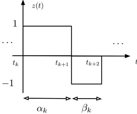
Figure 2: Duty-cycle modulation.
