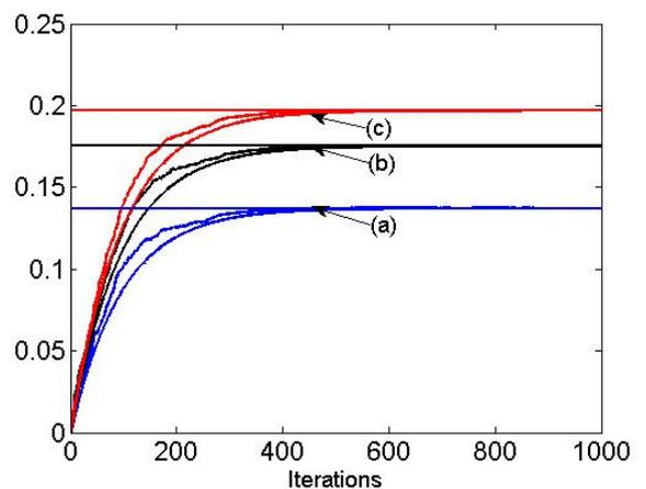
Figure 3 – Mean weight behavior for  $P=2$  and  $\alpha=0.4$ . Simulations (ragged) and model (continuous). (a) coefficient 20; (b) coefficient 40; (c) coefficient 30. Horizontal lines represent the true values of the plant coefficients.
