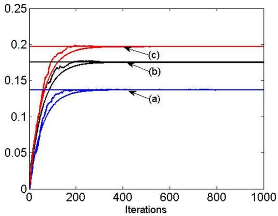
Figure 5 – Mean weight behavior for  $P=2$  and  $\alpha=0.9$ . Simulations (ragged) and model (continuous). (a) coefficient 20; (b) coefficient 40; (c) coefficient 30. Horizontal lines represent the true values of the plant coefficients.
