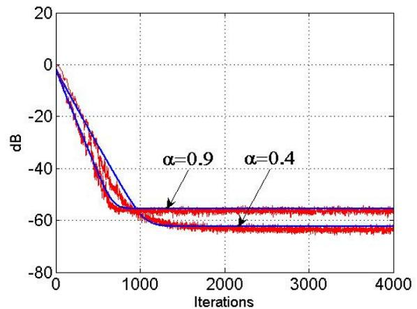
Figure 2 – Excess mean square error for  $P=4$ . Simulations (ragged - red) and model (continuous - blue).
