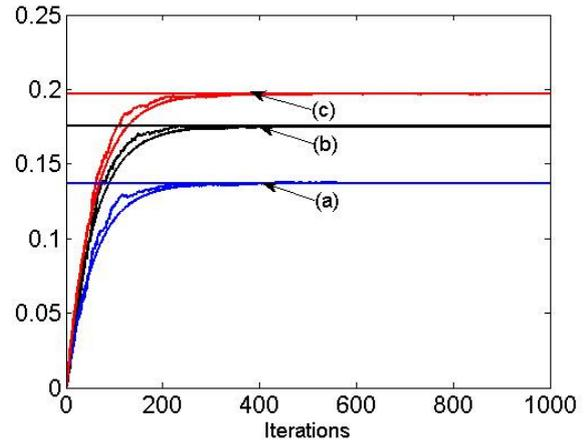
Figure 6 – Mean weight behavior for  $P=4$  and  $\alpha=0.9$ . Simulations (ragged) and model (continuous). (a) coefficient 20; (b) coefficient 40; (c) coefficient 30. Horizontal lines represent the true values of the plant coefficients.
