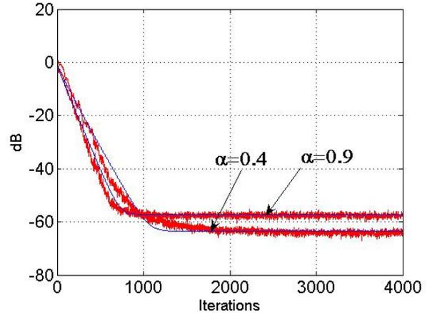
Figure 1 – Excess mean square error for  $P=2$ . Simulations (ragged - red) and model (continuous - blue).
