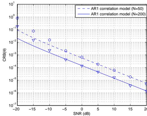
Fig.5 Exact CRB( $\theta$ ) for the AR1 correlation model and estimated MSE  $E(\hat{\theta}_{ML} - \theta)^2$  given by the ML estimator versus SNR for two values of  $N$  with  $f_d T = 0.01$ .
