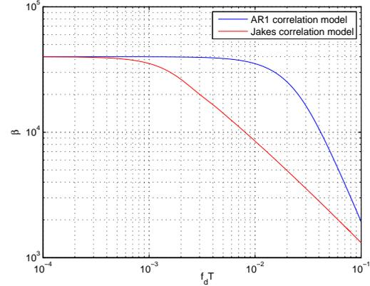
Fig.1 The channel-dependent parameter  $\beta$  for the Jakes and AR1 correlation model versus  $f_d T$  with  $N = 200$ .
