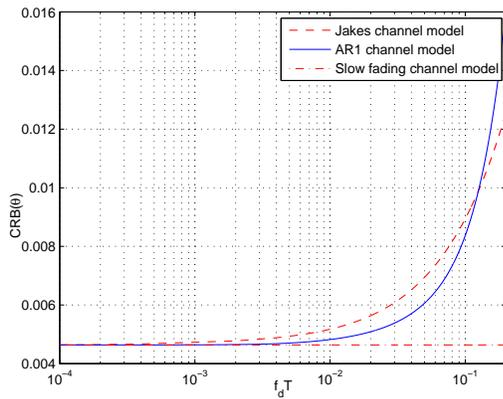
Fig.4 Exact CRB( $\theta$ ) for the Jakes and AR1 correlation model, and CRB<sup>Slow</sup>( $\theta$ ) versus  $f_d T$  with SNR = -15dB and  $N = 200$ .
