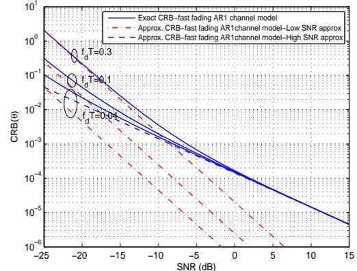
Fig.3 Exact CRB and its approximations for the fast fading AR1 correlation model for three values of  $f_d T$  versus SNR with  $N = 200$ .
