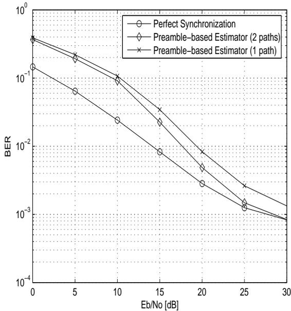
Figure 3: BER of the proposed joint estimator in multipath channel.
