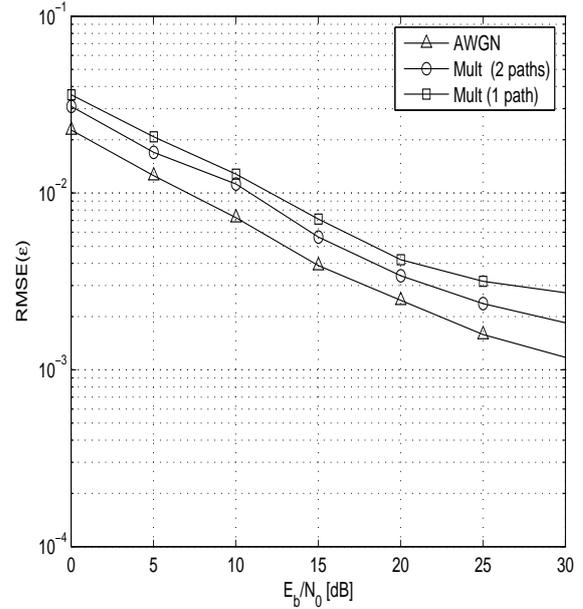
Figure 2: Performance of the proposed AML CFO estimator in AWGN and multipath channel.
