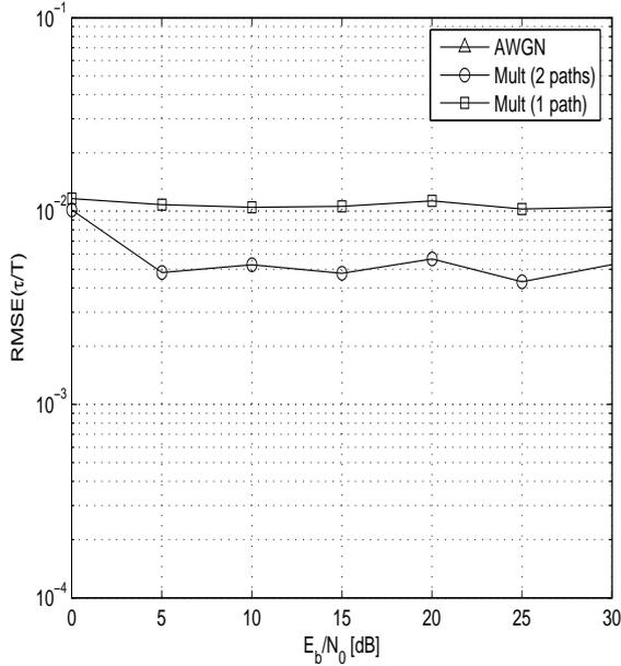
Figure 1: Performance of the proposed AML symbol timing estimator in AWGN and multipath channel.
