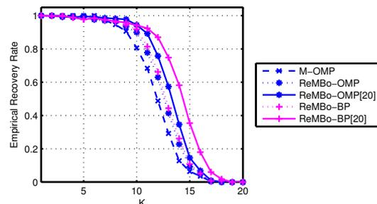
**Fig. 2:** A comparison between M-OMP and ReMBo-derived methods.
