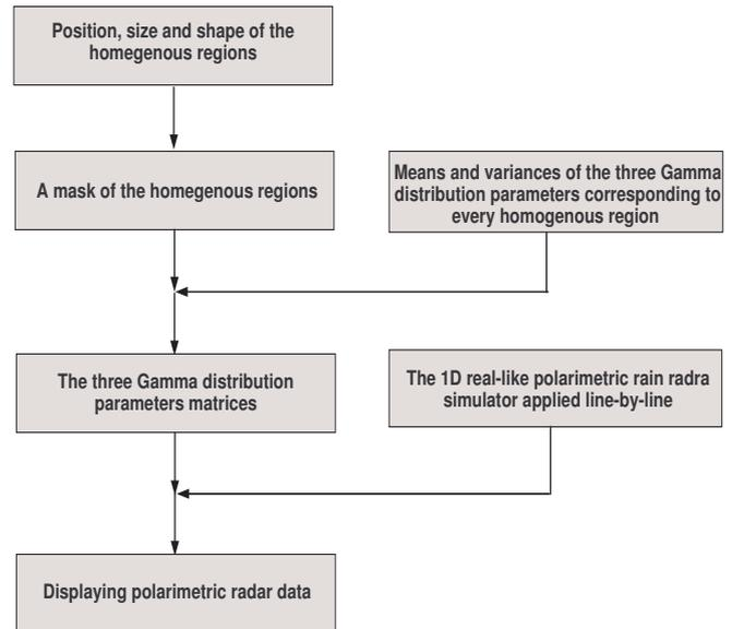
Figure 3: 2D Real-like radar Data simulator principal.
