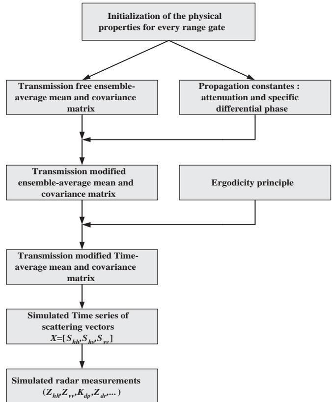
Figure 1: 1D Real-like radar Data simulator principal.
