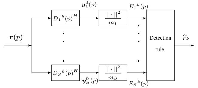
Figure 1: Block scheme of the proposed receiver.
