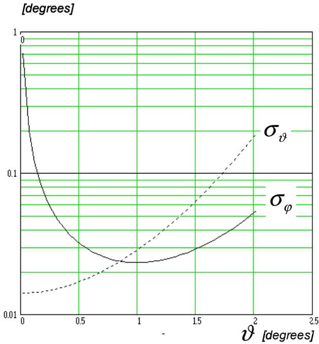
**Figure 1.** Asymptotic standard deviation  $\sigma_{\vartheta} = \sqrt{2}\beta\sigma_{\gamma}$  of the off-boresight angle estimate and  $\sigma_{\varphi}$  of the revolution angle estimates as a function of the off-boresight angle of the source.  $\beta = 1.0$  degree;  $\rho = 40$  dB.
