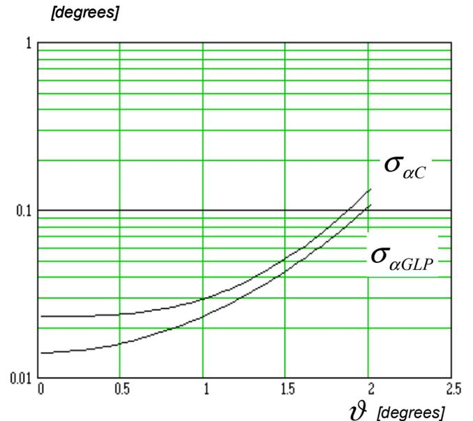
**Figure 3:** Asymptotic standard deviation of the error angle in azimuth for the radial trajectory  $\varphi_0 = 0$  degrees.  $\rho = 40$  dB.
