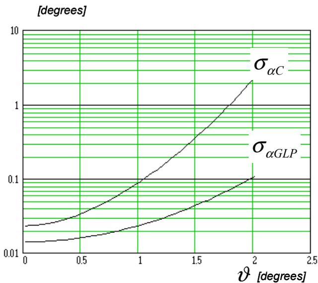
**Figure 5: Asymptotic standard deviation of the error angle in azimuth for the radial trajectory  $\varphi_0 = 90$  degrees.  $\rho = 40$  dB.**
