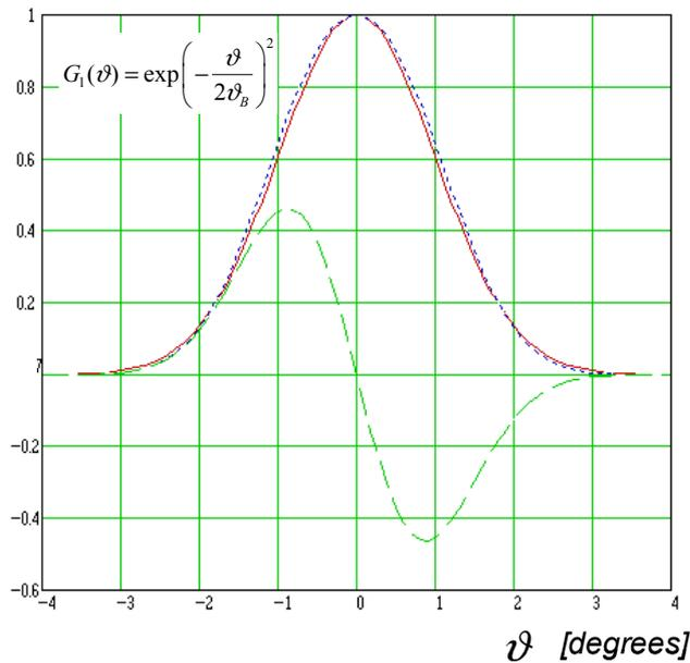
**Figure 2:** Comparison of the beams – Beamwidth of the GLP-ACM estimator:  $\beta = 1.0$  deg.; beam-width of the C-ACM monopulse estimator  $\beta_C = 0.8$  deg; beam displacement  $\alpha_0 = \gamma_0 = 0.7\beta_C$ .
