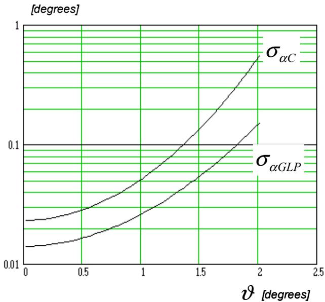
**Figure 4: Asymptotic standard deviation of the error angle in azimuth for the radial trajectory  $\varphi_0 = 45$  degrees.  $\rho = 40$  dB.**
