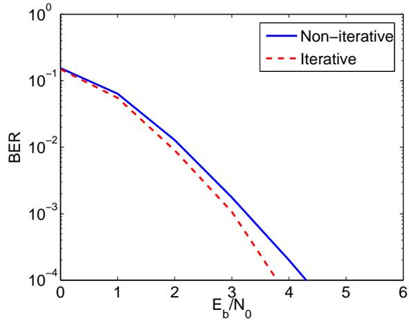
Figure 3: Performance of QPSK non iterative and iterative MC-CDMA receiver on reference channel 1
