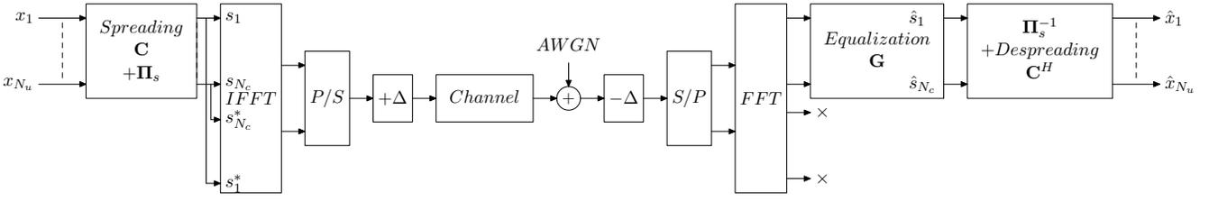
Figure 1: Modulator and demodulator of a MC-CDMA system in a PLC transmission
