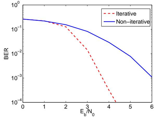
Figure 4: Performance of QPSK non iterative and iterative MC-CDMA receiver on reference channel 4
