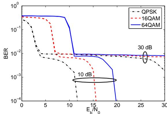
Figure 5: Performance of QPSK, 16QAM and 64QAM iterative MC-CDMA receiver on reference channel 4 with 1% impulse noise 10 dB and 30 dB higher than AWGN without interleaving
