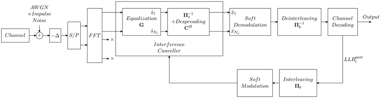
Figure 2: Iterative receiver of a MC-CDMA system in a PLC transmission
