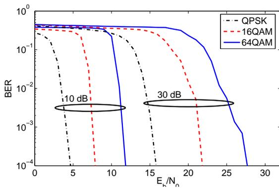
Figure 6: Performance of QPSK, 16QAM and 64QAM iterative MC-CDMA receiver on reference channel 4 with 1% impulse noise 10 dB and 30 dB higher than AWGN with interleaving
