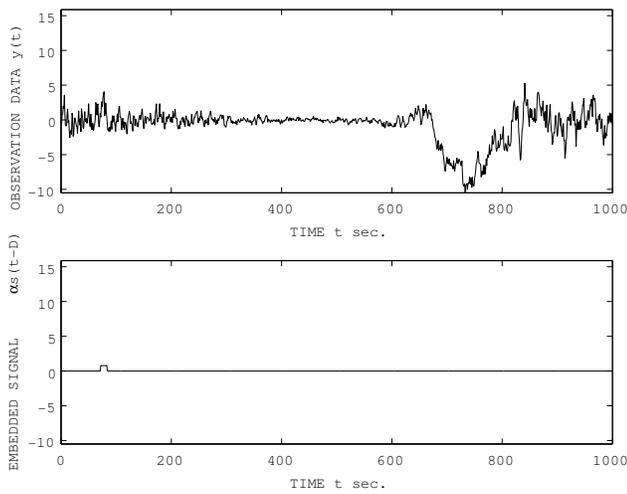
Fig. 4. A sample path of the observation data  $y(t)$  (top) and the embedded pulse signal  $s(t)$  (bottom).
