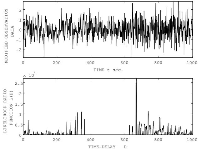
Fig. 3. The stationarized observation data  $\hat{y}_t$  (top) and the log-likelihood ratio function  $L(w; D)$  (bottom).
