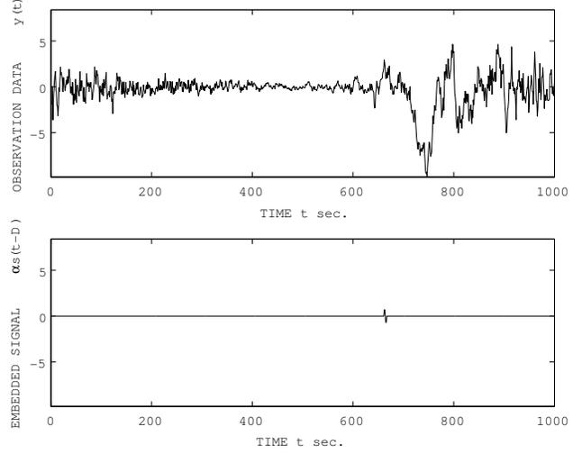
Fig. 1. A sample path of the observation data  $y(t)$  (top) and the embedded one-cycle sinusoidal signal  $s(t)$  (bottom).
