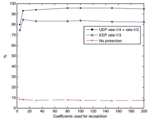
Fig. 7. Recognition rates for Rayleigh fading,  $E_b/N_0 = 3$  dB.
