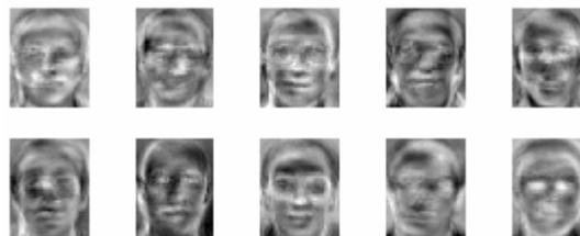
Fig. 3. Eigenfaces with the highest eigenvalues.
