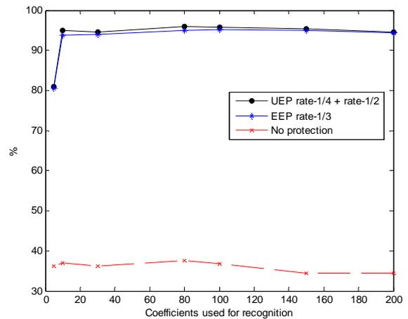
Fig. 5. Recognition rates for AWGN at  $E_b/N_0 = 3$  dB.
