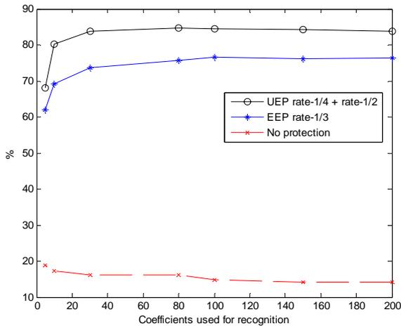
Fig. 4. Recognition rates for AWGN channel,  $E_b/N_0 = 0$  dB.
