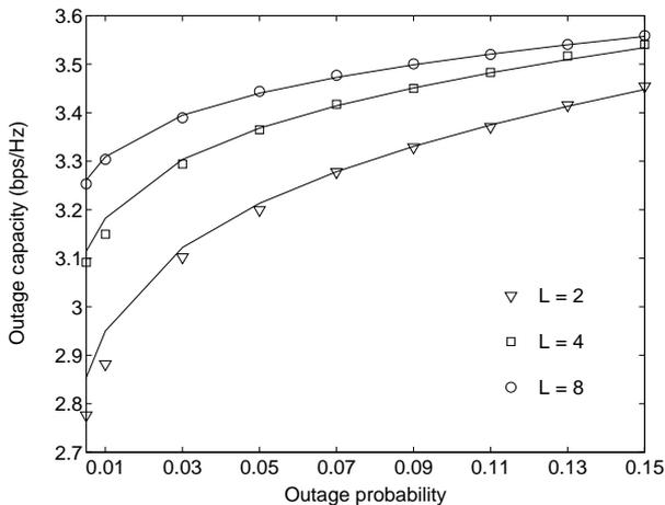
**Fig. 2.** Outage capacity of a  $3 \times 3$  OFDM-STBC system, as a function of the outage probability, for different channel lengths.
