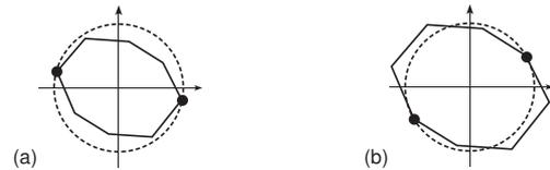
Figure 1: Principal signals and the MAP defining polytope. The dotted circles denote the unit sphere in 2D signal space. The two polygons are different scales of the same MAP defining polytope. (a) A principal signal, obtained at a vertex of the defining polytope. (b) A vertex which does not represent a principal signal.
