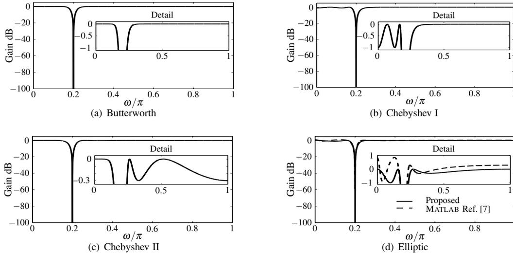
Figure 2: Magnitude responses of the designed filters.
