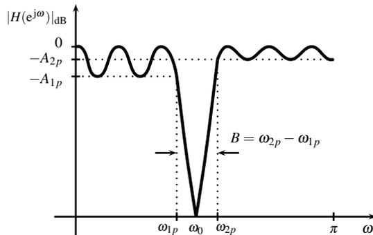
Figure 1: Gain characteristic of a notch filter.
