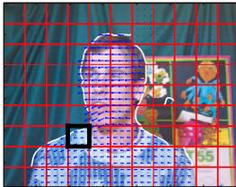
Figure 5: Macroblock spline segmentation with occlusions management
