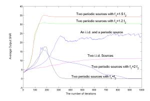
Figure 3: A comparison between the SNR of the gradient method in separation of two sources with 4 different cases of inputs: two i.i.d. sources, a periodic source and an i.i.d. one, two periodic sources with integer or non-integer ratio of the main frequencies  $f_1$  and  $f_2$
