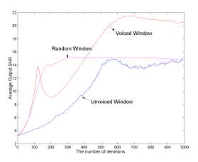
Figure 8: performance of the gradient method on different cases of the two speech sources: Voiced-Voiced, Voiced-Unvoiced, Unvoiced-Unvoiced and random selection of buffered samples (average of 20 random selection).
