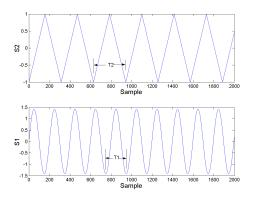
Figure 2: 1500 sample from two periodic sources, a sinuous and a sawtooth with periods  $T_1$  and  $T_2$
