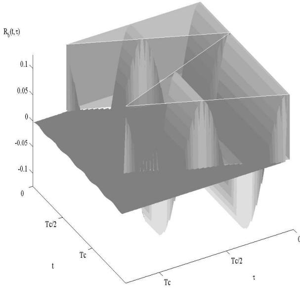
Figure 2: The time varying autocorrelation,  $R_b(t, \tau)$ , of a binary phase shift keying modulation.  $T_c$  is the rectangular pulse width. The carrier frequency,  $f_0$ , is equal to  $1/33 \cdot f_s$ , with  $f_s$  the sampling frequency.
