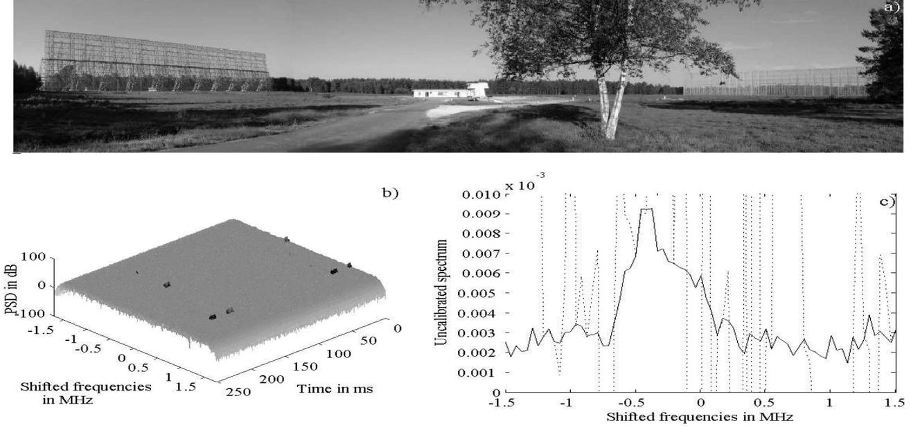
Figure 1: Detection and blanking scheme applied on the III Zw 35 observations. **(a)** The decimeter radio telescope of Nançay. **(b)** Time-frequency (t-f) representation of the observations. Some of the t-f slots used by the Iridium constellation satellites are clearly visible. III Zw 35 source is scrambled by the RFI. **(c)** Normalized averaged spectrum without (dashed line) and with (continuous line) blanking. The receiver filter shape has been subtracted.
