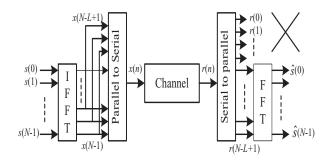
Figure 1: A basic baseband OFDM system, transmitting subsequent blocks of *N* complex data.
