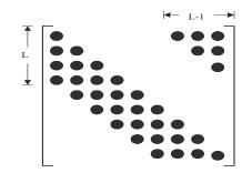
Figure 2: Diagonal structure of the time-domain CCM H.
