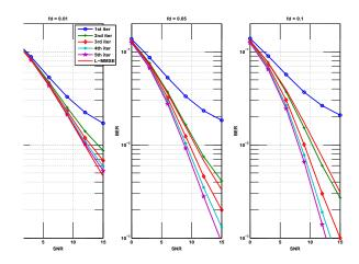
Figure 3: Comparison of BER performance of MMSEiterative algorithm with the L-MMSE equalizer up to five iterations and at different DS.
