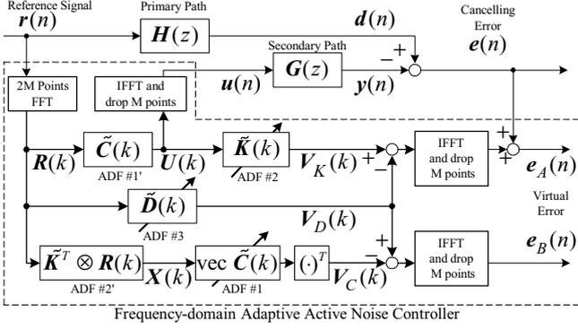
Figure 2: Freq.-domain algorithm for multichannel ANC
