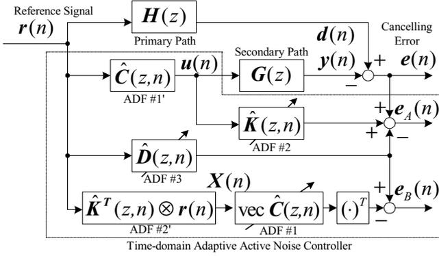
Figure 1: Time-domain algorithm for multichannel ANC
