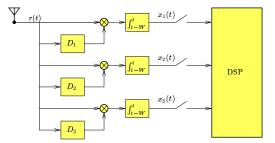
Figure 1: The structure of the autocorrelation receiver.
