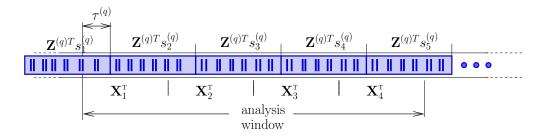
Figure 2: The structure of analysis window for the asynchronous TR-UWB scheme.
