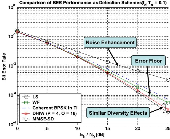
Figure 5: The comparison of average BER performance ; least square(LS), Wiener filter(WF), coherent BPSK in time-invariant channels(TI), Doppler diversity technique with hybrid interference cancellation and Wiener filter(DHIW), minimum mean square error with successive detection(MMSE-SD) ( $N = 64$ ,  $P$  : a number of sub-carriers detected at each stage,  $Q$  : total number of stages,  $f_d T_s$  : normalized Doppler frequency)
