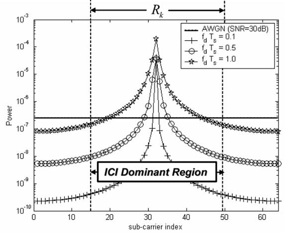
Figure 4: The ICI distribution to the  $k$ th sub-carrier in time-varying multipath channels ( $k = 32$  : the index of the ICI-corrupted sub-carrier,  $f_d T_s$  : normalized Doppler frequency)
