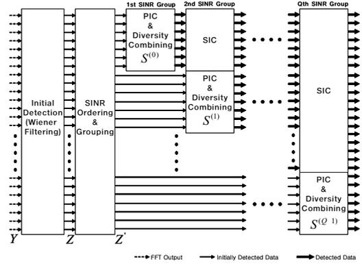
Figure 2: The block diagram of Doppler diversity technique with hybrid interference cancellation and Wiener filter (DHIW)
