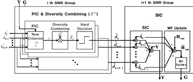
Figure 3: A block diagram of the HIC block using a new criterion
