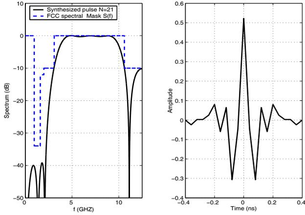
Figure 3: For  $N = 21$ , optimally designed pulse shaper and its FT for  $\alpha = 9.32 \cdot 10^9$  and  $L = 10$ .
