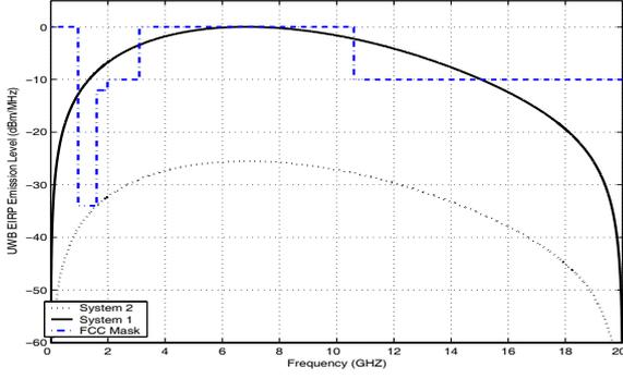
Figure 1: The power spectral density of the Gaussian monocycle pulse for the tow peak amplitude  $A_1$  and  $A_2$  and the FCC indoor spectral emission mask
