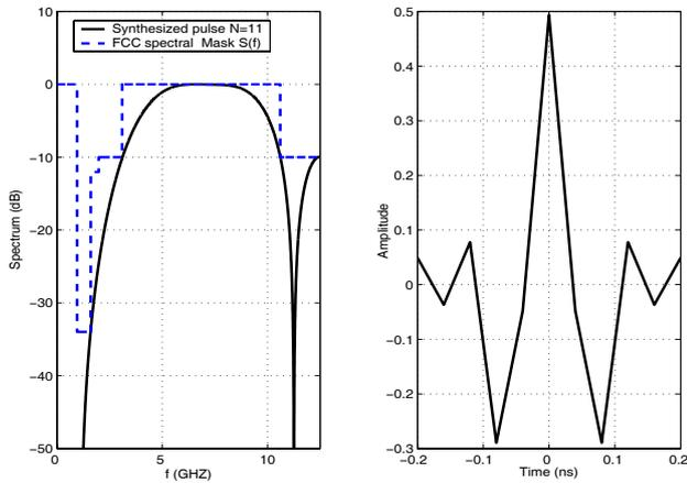
Figure 4: For  $N = 11$ , optimally designed pulse shaper and its FT for  $\alpha = 12.26 \cdot 10^9$  and  $L = 10$ .
