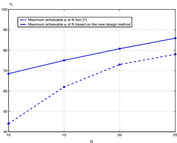
Figure 5: Evolution of the maximum normalized effective signal power versus the pulse duration.
