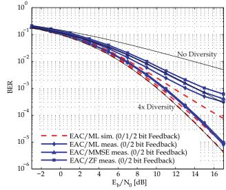
Figure 5: Different receivers for the EAC (QAM, 4.17 MSymbols/s)
