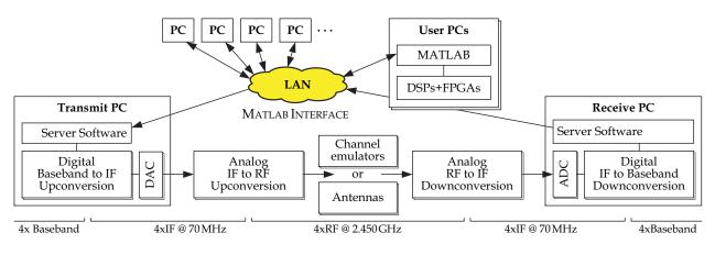
Figure 1: Measurement setup.
