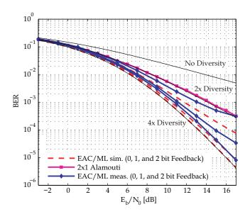
Figure 4: Comparison AC/EAC, measured and simulated (QAM, 4.17MSymbols/s)
