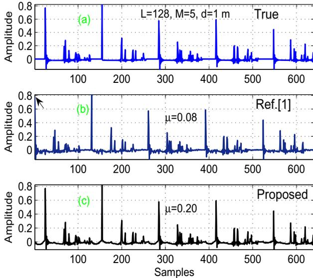
Figure 2: Results on channel estimation at SNR=20 dB using the NMCFLMS.
