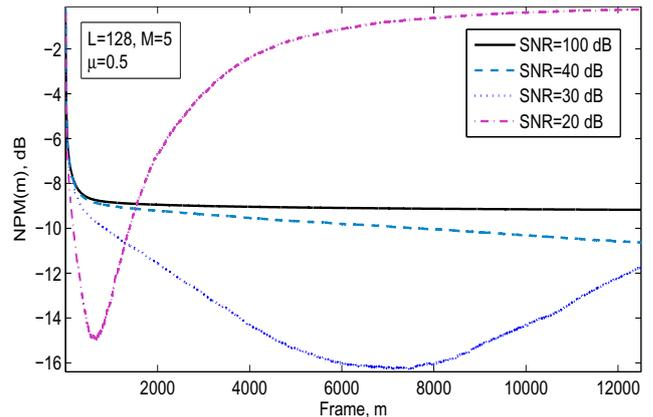
Figure 1: Variation of NPM with iteration at different SNRs for  $\mu = 0.5$ . The array consists of  $M = 5$  microphones, source-mic separation  $d = 1m$ , and the length of the channel impulse response is  $L = 128$ .
