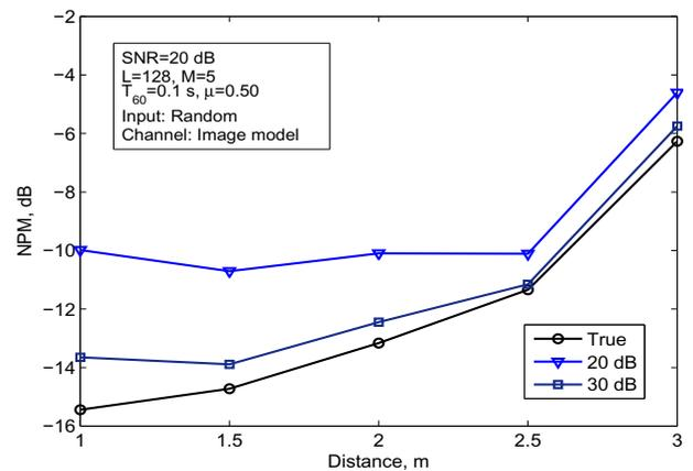
Figure 4: Final value of NPM as the source moves away from the microphone array at SNR=20 dB. The array consists of  $M = 5$  microphones and the length of the channel impulse response is  $L = 128$ .
