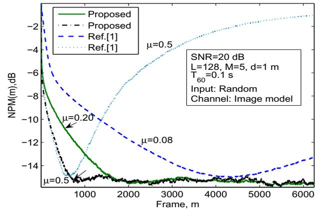
Figure 3: Variation of NPM with iteration at SNR=20 dB. The array consists of  $M = 5$  microphones, source-mic separation  $d = 1m$ , and the length of the channel impulse response is  $L = 128$ .
