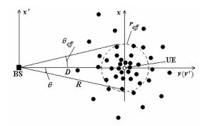
Figure 1 Illustration of the Gaussian channel model
