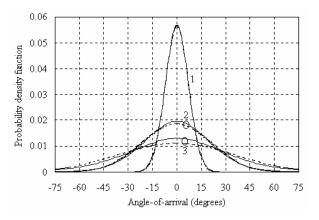
Figure 2 PDF of the AoA of the multipaths at the BS. The angle spread  $\Delta$  (where  $\Delta = 2\theta_{eff}$ ) is equal to 20, 60 and 100 degrees (curves 1,2,3 respectively). The solid and dashed curves correspond to the exact formula (8) and its Gaussian approximation (9) respectively.
