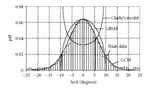
Figure 3 The PDFs for the AoA of the multipath components at the BS for GCM, GBSBM and Clarke's models and for the measured histograms.
