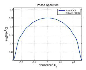
Figure 2: Phase response of the designed 1-D seismic migration filter using pure POCS (solid line) and relaxed POCS (dashed line) with N = 39,  $k_{c_p} = 0.25$ ,  $k_{c_s} = 0.3347$ ,  $\delta_p = \delta_s = 10^{-3}$ , and  $\varepsilon = 10^{-12}$ .
