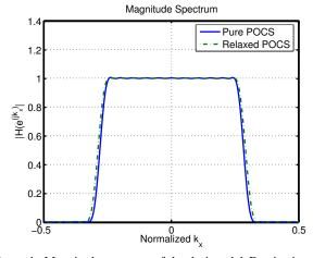
Figure 1: Magnitude response of the designed 1-D seismic migration filter using pure POCS (solid line) and relaxed POCS (dashed line) with N = 39,  $k_{c_p} = 0.25$ ,  $k_{c_s} = 0.3347$ ,  $\delta_p = \delta_s = 10^{-3}$ , and  $\varepsilon = 10^{-12}$ .
