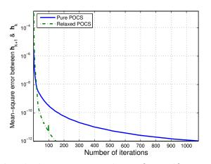
Figure 3: The mean-square error between  $\mathbf{h}_{k+1}$  and  $\mathbf{h}_k$ , versus the number of iterations, for the designed 1-D seismic migration filter using pure POCS and relaxed POCS with N = 39,  $k_{c_p} = 0.25$ ,  $k_{c_s} = 0.3347$ ,  $\delta_p = \delta_s = 10^{-3}$ , and  $\varepsilon = 10^{-12}$ .
