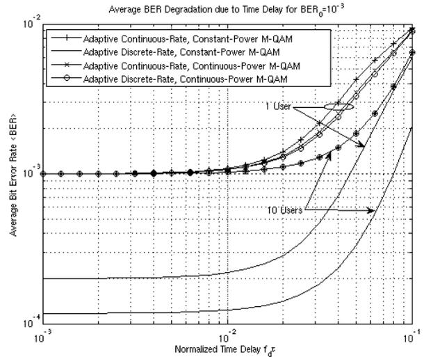
Figure 4: Average BER degradation due to time delay for ORRF using M-QAM rate adaptation with  $\bar{\gamma}=15$  dB, 5 fading regions and  $\text{BER}_0 = 10^{-3}$ .
