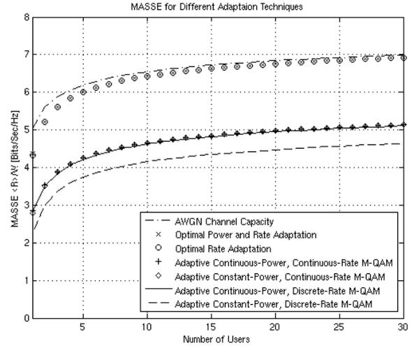
Figure 2: Maximum average system spectral efficiency for ORRF scheduling with  $\bar{\gamma}=15$  dB, 7 fading regions and  $\text{BER}_0 = 10^{-3}$ .
