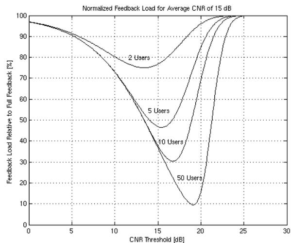
Figure 1: Normalized feedback load as a function of  $\gamma_{th}$  with  $\bar{\gamma} = 15$  dB.
