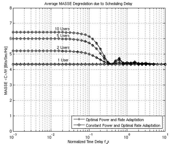
Figure 3: Average degradation in MASSE due to scheduling delay for ORRF using optimal power and rate adaptation and optimal rate adaptation.
