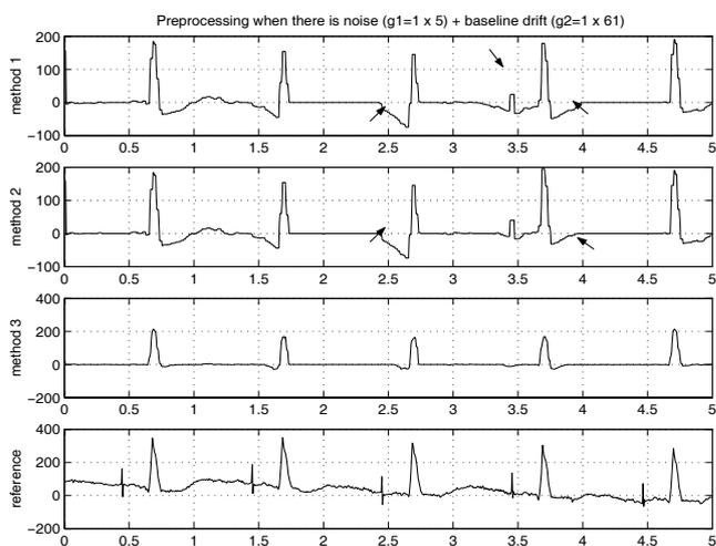
Figure 7: The preprocessing with three methods for removing high frequency noise at first and next, the baseline wander correction.
