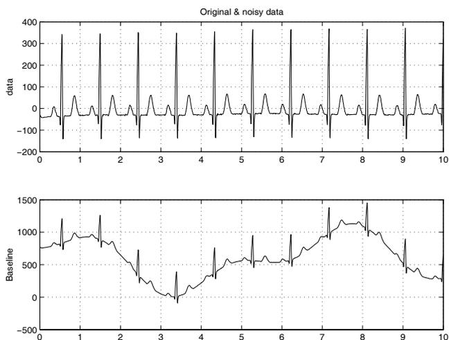
Figure 3: Original and (artificially) corrupted signal.
