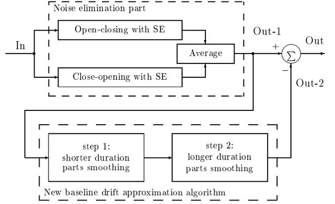
Figure 1: Simplified block diagram of ECG preprocessing (method 2).
