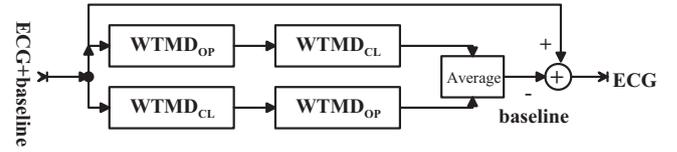
Figure 2: Block diagram of ECG preprocessing (the proposed method (3)).
