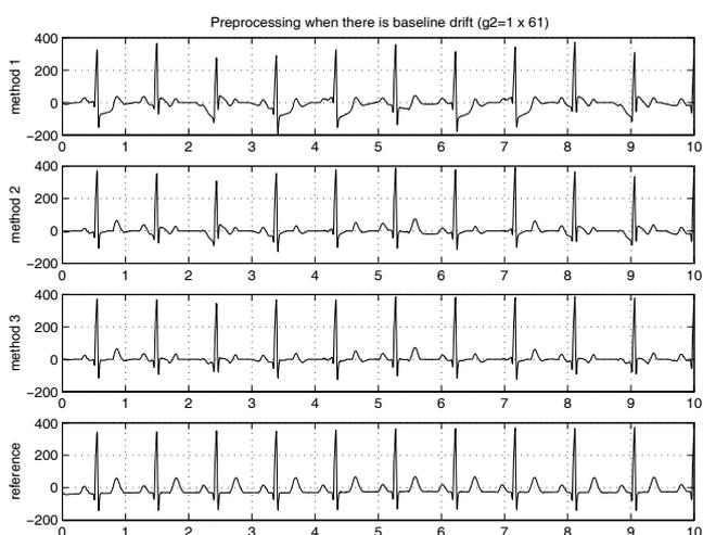
Figure 4: Baseline drift correction with three methods.
