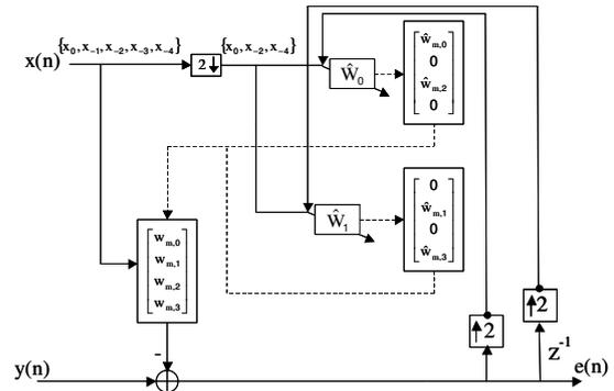
Figure 1: Block diagram of the S-NLMS for  $D = 2$ .
