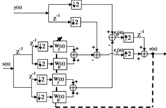
Figure 3: PR delay chain with polyphase filters adapted jointly.
