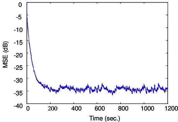
Figure 8: MSE convergence of the S-NLMS algorithm in time-domain for  $D = 1, 4, 8, 12$  and  $24$ , and stationary input signals.
