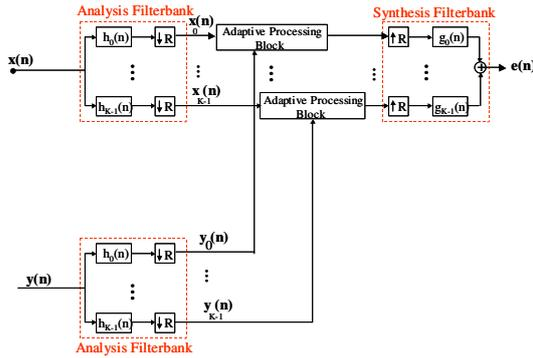
Figure 6: Block diagram of the OS-SAF system.
