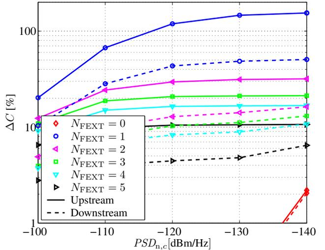
Figure 5: Capacity gain  $\Delta C$  versus CM background noise PSD level  $PSD_{n,c}$  for different numbers  $N_{\text{FEXT}}$  of FEXT disturbers in upstream (solid lines) and downstream (dashed lines) direction ( $PSD_{n,d} = -130\text{dBm/Hz}$ ,  $L_{\text{loop}} = 1000\text{m}$ ,  $L_{\text{xt}} = 100\text{m}$ ).
