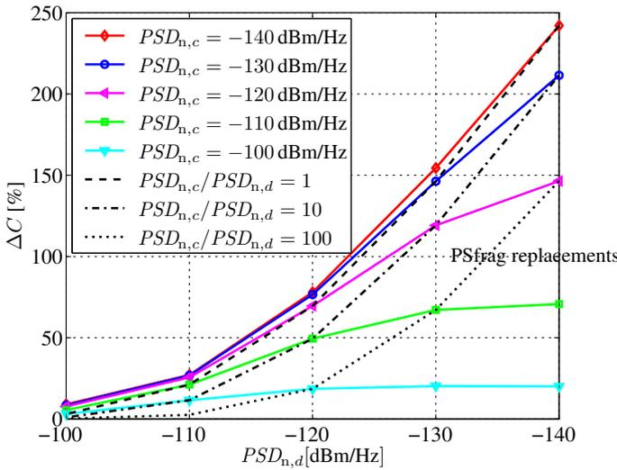
Figure 3: Capacity gain  $\Delta C$  as a function of the background noise PSD levels  $PSD_{n,d}$  at the DM port and  $PSD_{n,c}$  at the CM port in *upstream* direction for a 0.6mm loop of length  $L_{\text{loop}} = 1000\text{m}$  with a single equal-power FEXT disturber ( $N_{\text{FEXT}} = 1$ ) located at a distance  $L_{\text{xt}} = 100\text{m}$ . The non-solid lines show the capacity gains for constant ratios  $PSD_{n,c}/PSD_{n,d}$ .
