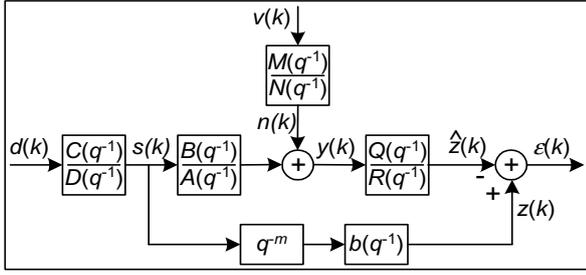
Figure 1: Channel shortening model employing an IIR shortening filter to approximate an IIR channel to a finite length target impulse response. The channel input  $s(k)$  and the noise  $n(k)$  are ARMA processes.
