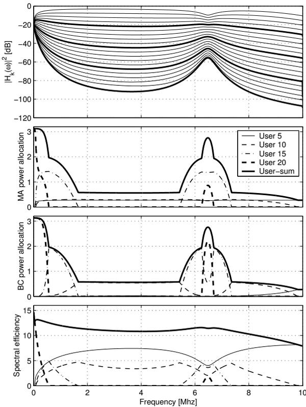
Figure 3: Channel frequency responses ( $K = 20$  users), power allocations and spectral efficiency for  $S_4 = \{5, 10, 15, 20\}$
