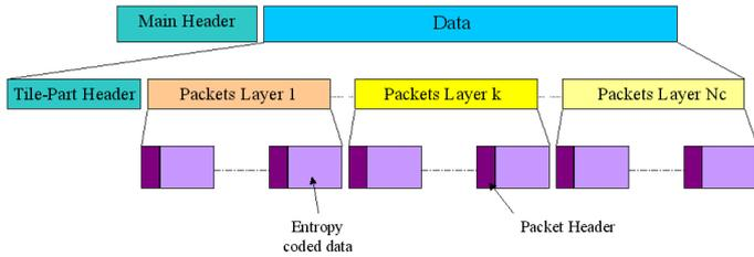
Figure 3: JPEG2000 Syntax for  $N_c$  Quality layers configuration.
