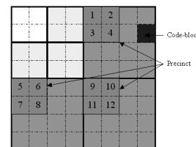
Figure 2: Code-blocks and Precincts for a 3 resolution levels wavelet transform of a tile.
