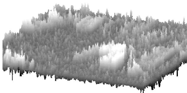
**Figure 2a:** a DEM obtained from a classical interferometric technique on a semi-built-up area.
