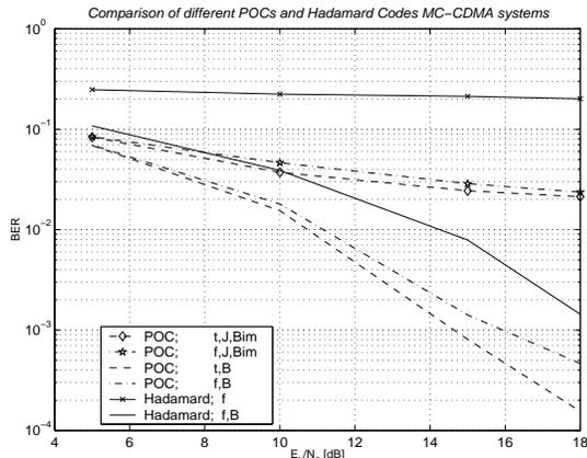
Fig. 2. MC-CDMA schemes with different noise levels
