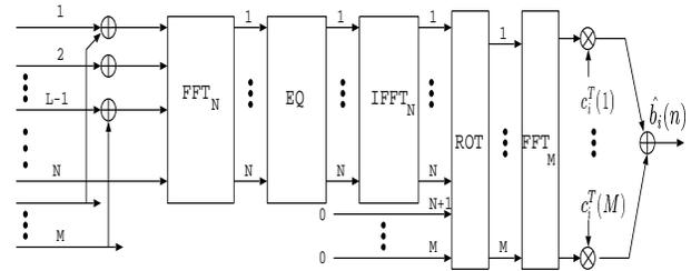
Fig. 1. Frequency equalizer
