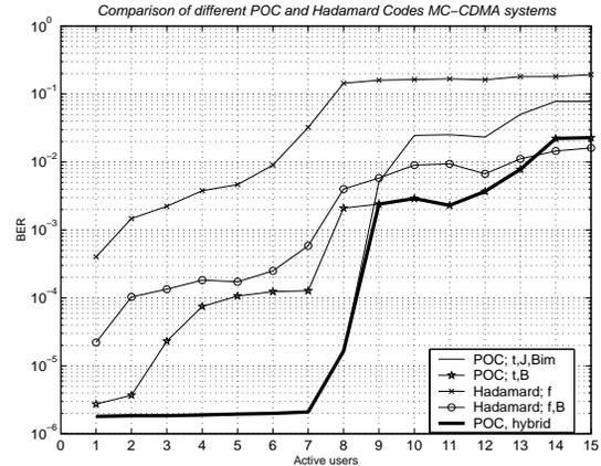
Fig. 3. MC-CDMA with different number of active users
