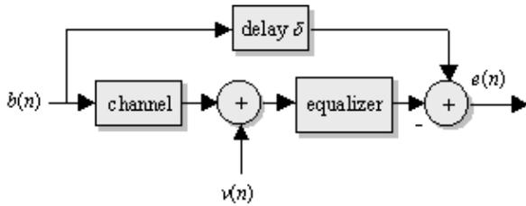
Figure 3: Block diagram of equalization scheme.
