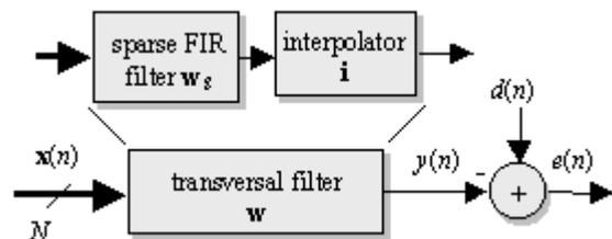
Figure 1: Interpolated Wiener filtering
