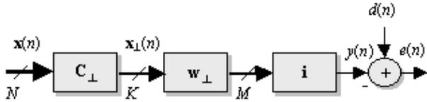
Figure 2: GSC structure for interpolated Wiener filtering.
