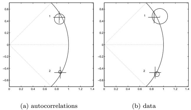
Figure 3: Positions and variances of the estimated poles. (a)  $L = 23$ ,  $p = 10$  and  $c = 20$ , (b)  $p = 10$  and  $c = 20$ .
