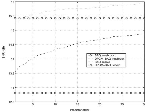
Figure 4: BAQ and DPCM-BAQ performance (azimuth) at 3 bit/sample for *Jesolo* and *Innsbruck*
