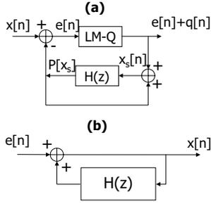
Figure 1: (a) DPCM encoder with Lloyd-Max quantizer in the feedback loop; (b) DPCM decoder with inverse prediction error filter
