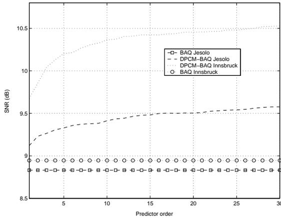
Figure 5: BAQ and DPCM-BAQ performance (azimuth) at 2 bit/sample for *Jesolo* and *Innsbruck*
