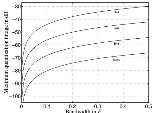
Fig. 4. Relationship between the input bandwidth and the attenuation of the first quantization image.
