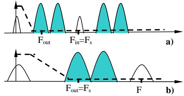
Fig. 6. Input signal spectrum and the anti-aliasing filter defined in terms of the (a) input and (b) output sampling interval.
