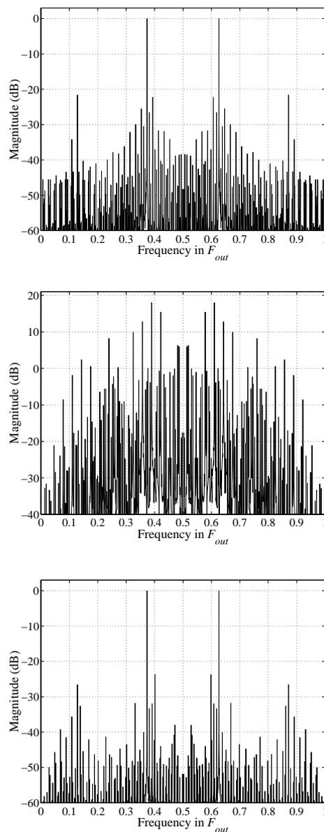
Fig. 7. The output spectrum for the modified Farrow structure for (a)  $B=1$ , trasposed Farrow structure for (b)  $B=1$ , and (c)  $B=7$  bits.
