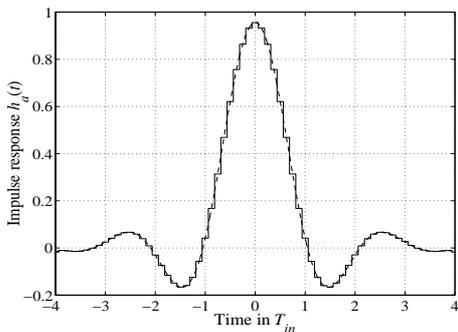
Fig. 2. Impulse response of the interpolation filter for unquantized (dashed line) and quantized (solid line) fractional interval, with  $B=3$ .
