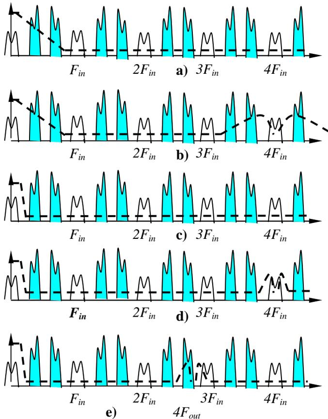
Fig. 5. SRC with anti-imaging filter with (a) high precision and (b) finite precision of 2 bits; SRC with anti-aliasing filter with (c) high precision, (d) finite precision of 2 bits, and (e) when  $\mu$  is defined in terms of  $T_{out}$ .
