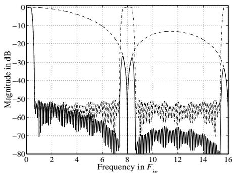
Fig. 3. The frequency response of the example interpolation filter when  $\mu_1$  is quantized to  $B=3$  bits.
