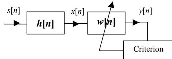
Figure 1. Schematic diagram of blind deconvolution
