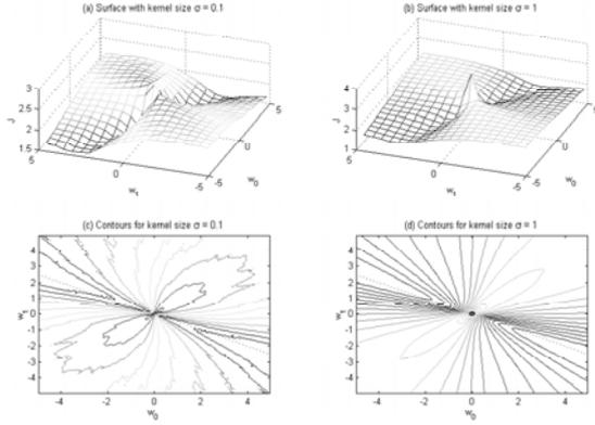
Figure 2. Illustration of the performance surface and its contour lines for a 2-tap deconvolving filter case using two different kernel size values in the entropy estimator.
